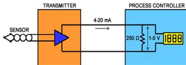
The precision resistor converts the 4-20 mA signal from the transmitter to a voltage drop, which is compatible with the data processing components. Normally, the resistor is contained in the input circuitry of the data processing equipment.
