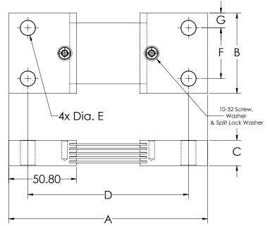
\*Dimension tolerances: ±0.381mm for hole diameters. All other dimensions have a ±0.762mm tolerance
